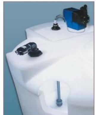
Assmann Corporation advises that using its Double Wall Tank system with a bottom sidewall fitting may not meet local codes for secondary containment, as tank contents could escape containment area in the event of fitting damage. Assmann recommends that its Double Wall Tanks be fitted with a top suction line and foot valve to provide constant flow to the pump.
