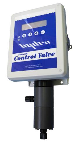
By replacing rotating assemblies with a simple linear design and incorporating a lengthened V-notch stem, the Hydro Instruments CV-230 Control Valve produces precise and repeatable feed rate control with minimal wear.
