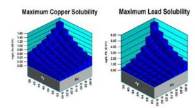
Sample + Analyze = Custom Treatment WatSim allows a water treatment chemist to evaluate the scale and corrosion potential for common scalants over the range of water chemistry, temperature, and pH anticipated in a system.
